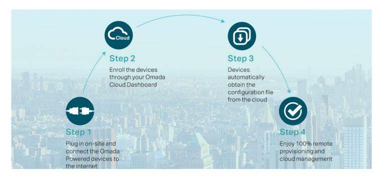
1. Zero-Touch Provisioning is supported when using Omada Cloud-Based Controller
